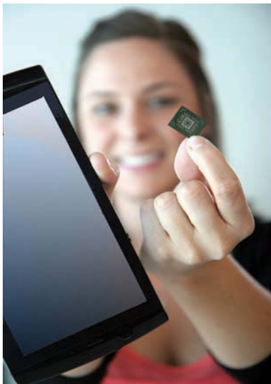
Figure 4 SanDisk's integrated solid-state drive offers fast, lightweight, and affordable storage for smartbooks, ultrathin PCs, and tablets.
