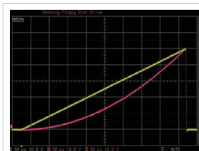
Figure 2 At the midwidth of the pulse, the quadratic parabolic pulse's voltage level (pink trace) is exactly one-fourth of its peak level.
