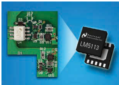
This 180W, one-eighth-brick, fully regulated converter demonstrates the system-performance advantages of coupling eGaN FETs with the LM5113 driver (courtesy National Semiconductor).
